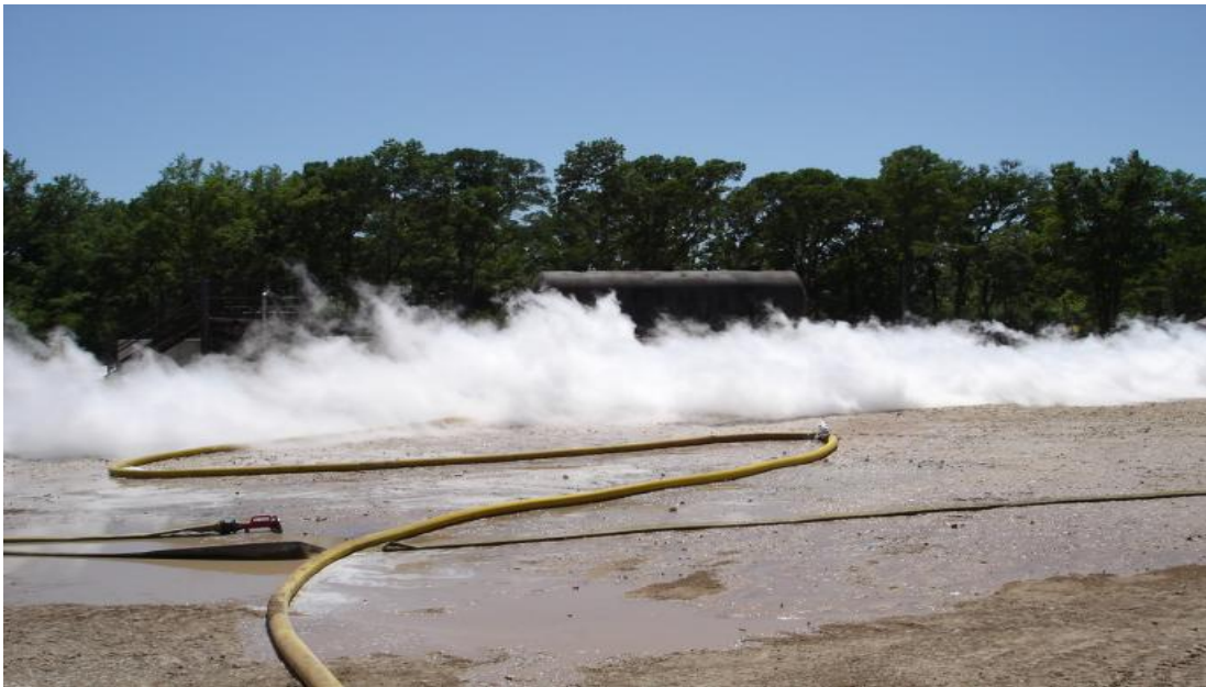
Figure 4: Controlled release of LNG for the purpose of staff training [8]
