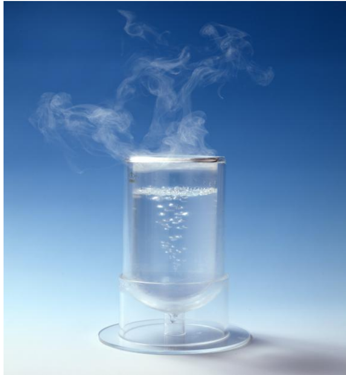
Figure 3: LNG at room temperature [8]
